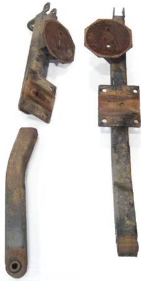
The stock trailing arms on the Monaco Gold suspension used on Roadmaster R4R and RR4R chassis (above left) are smaller and reportedly more susceptible to failure than the more substantial trailing arms (above right) included in the TRA-1003 suspension kit from Source Manufacturing.
